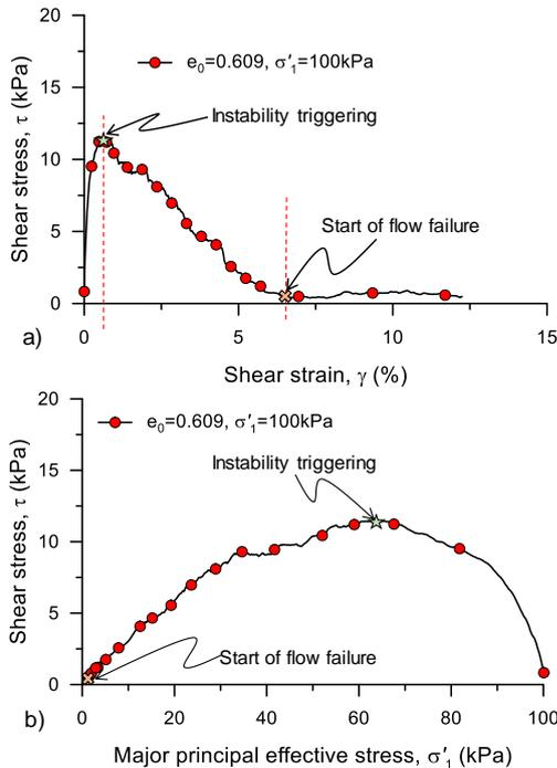
Figure 3. Constant volume behaviour under simple shear condition for flow behavior: (a)  $\tau$ - $\gamma$  and (b)  $\tau$ - $\sigma'_N$  spaces.
