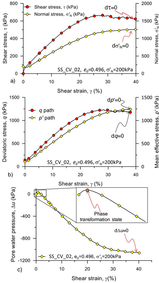
Figure 2. Constant volume behaviour under simple shear condition for non-flow behavior: (a)  $\tau$ - $\sigma'_N$ - $\gamma$ , (b)  $q$ - $p'$ - $\gamma$  and (c)  $\Delta u$ - $\gamma$  spaces.
